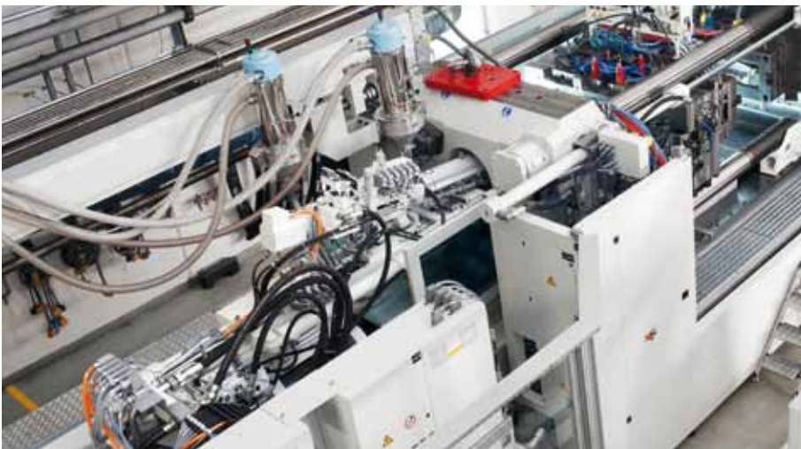
Due to their general design, the SpinForm machines provide sufficient room for even complex periphery and automation equipment to be easily integrated.
